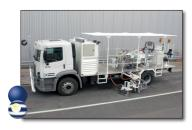
H37-1000P Combi roadmarking truck with pressurised containers (2 x 540 l) for cold paints and sprayable 2-comp. cold plastics, mixing ratio 98:2 using Airless method with path-dependent metering pump (AMAKOS®)
