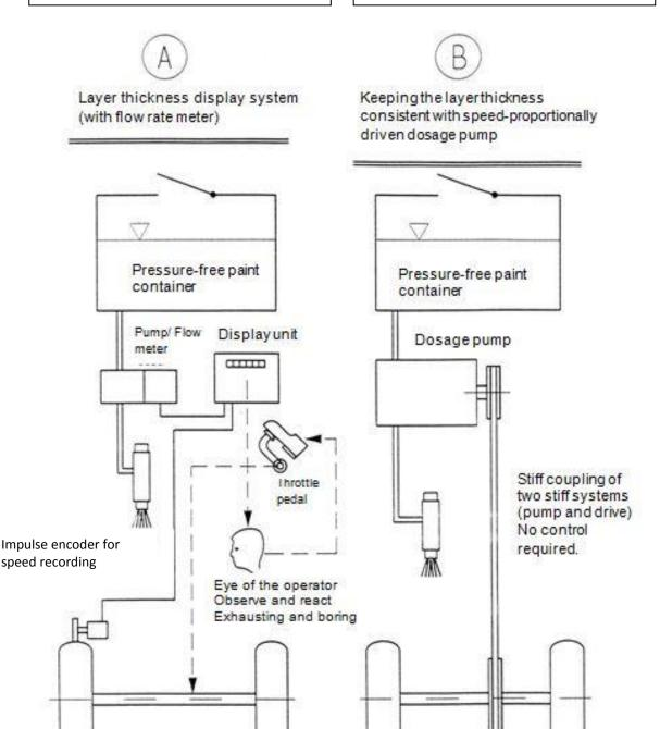
Display of the calculated averages of the layer thickness, display delayed Reactions of the operator to target-actual deviations delayed. Compensation of the target-actual deviation delayed. Large dependency on care and fatigue of the operator. Operator acts as controller. At target-actual deviation zero, the operating speed must <u>not</u> change. Any change leads to a layer thickness change in the opposite direction.
