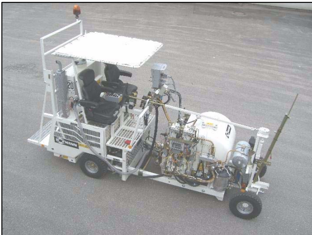
H18-1 equipped for the application of 2-component sprayable cold plastic (Airless) with mixing ratio 98:2
