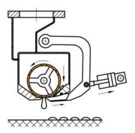
Execution of profiled markings (MultiDotLine®) with a lowered drum. The profile drum is thereby slightly pressed onto an edge of carbide metal, cleanly separating the individual material portions – the secret of unbeatable clean material dots!
