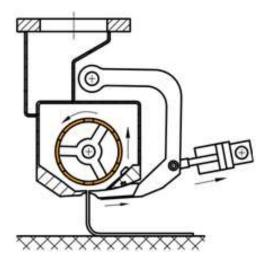
Executing plain line markings with raised drum. Drum can be pneumatically lowered and raised during the marking operation by the operator.
