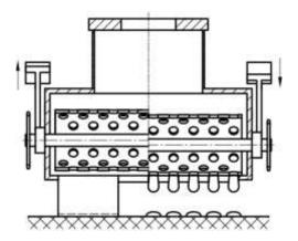
Rotation of an hollow cylinder with openings (profile drum) inside of the extruder housing.
