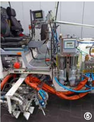
Metering process: Plunger pump for 98% main component as well as for 2% hardener component, for sprayable 2c cold plastics Airspray (low pressure method) with MALCON4E
