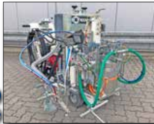
H9-1 Airless 2c M98:2 equipped for Airless (high pressure spraying method), 1-component cold paints as well as sprayable 2-component cold plastics, with mixing ratio 98:2
