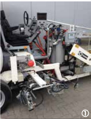
Metering process: Bellow pump for spray-able thermoplastics with MALCON4E
