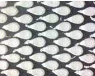
Drum rotating in driving direction ⇒ drop shaped pattern
