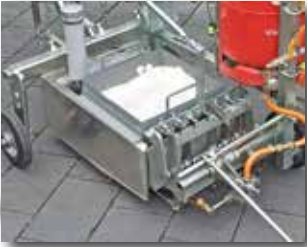
RP30 – Thermoplastic screed box with set of shutters for line widths up to 30 cm
