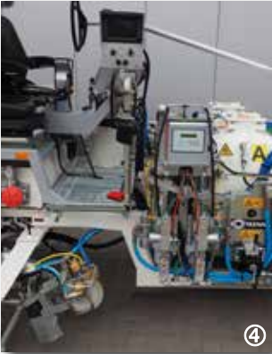
Metering process: Plunger pump for 98% main component as well for 2% hardener component, for sprayable 2c cold plastics Airless (high pressure method) with MALCON4E
