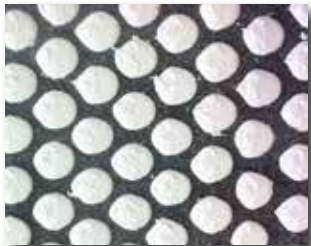
Drum rotating against driving direction ⇒ round pattern
