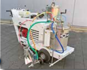
H9-1 Airspray (Low pressure spraying method)
