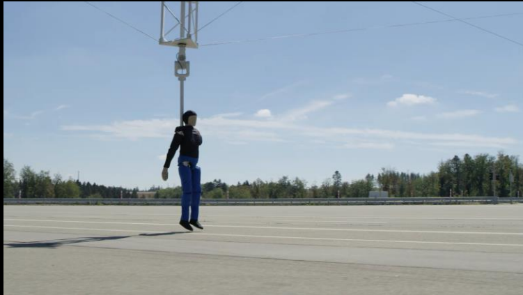
The 6D Target Mover in combination with the Active Safety Test Robot increases the realism of test scenarios.
