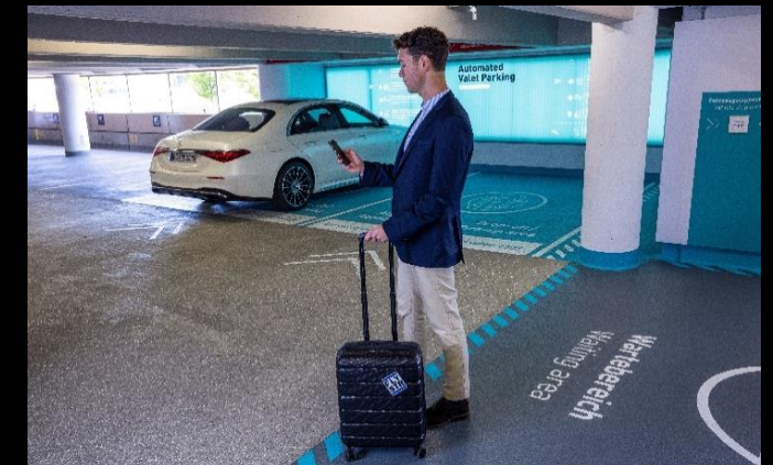
If specified with preinstallation for the INTELLIGENT PARKING PILOT, the S-Class (and EQS) is prepared for highly automated driverless parking (Automated Valet Parking, AVP, SAE Level 4) [12].
