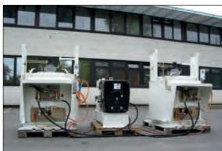
③ D350 Two D350 with propane gas burner, 10 kW power station
